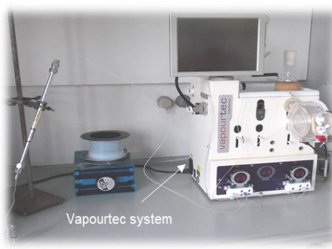
Figure 18. Solid-liquid asymmetric phase transfer benzylation of L-alanine imine in packed-bed reactors (streams delivered by a syringe pump (left) or by Vapourtec flow system (right))
