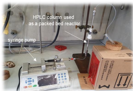
Figure 18. Solid-liquid asymmetric phase transfer benzylation of L-alanine imine in packed-bed reactors (streams delivered by a syringe pump (left) or by Vapourtec flow system (right))
