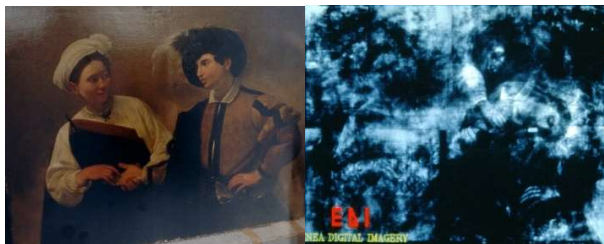
Figure 1. Radiography of the Caravaggio canvas “La buona ventura”. The underlayer is another painting. (measurements carried out by ENEA – National Agency for the Energy and the Environment)
