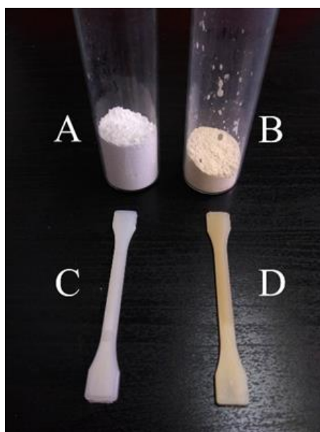
Figure 3.1 - Visual comparison of HNT s (A) and HNT H (B) and their respective composites prepared via injection moulding: PA6 melt _HNT s _4 (C) and PA6 melt _HNT H _4 (D).
