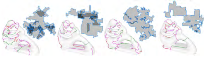
Fig. 5. Results of the initial cut selection procedure with different edge prioritization strategies: From left to right, the purely random selection of expansion moves, cut-straightening only, overlap avoidance only, and the combination of the two criteria, which we use in all other examples. In each case, we show the cut over the mesh Q . The approximated parametric space (with overlaps in darker grays – on the right, the patch boundary in 2D may appear artificially less straight due to the approximations of parametric position estimation).
