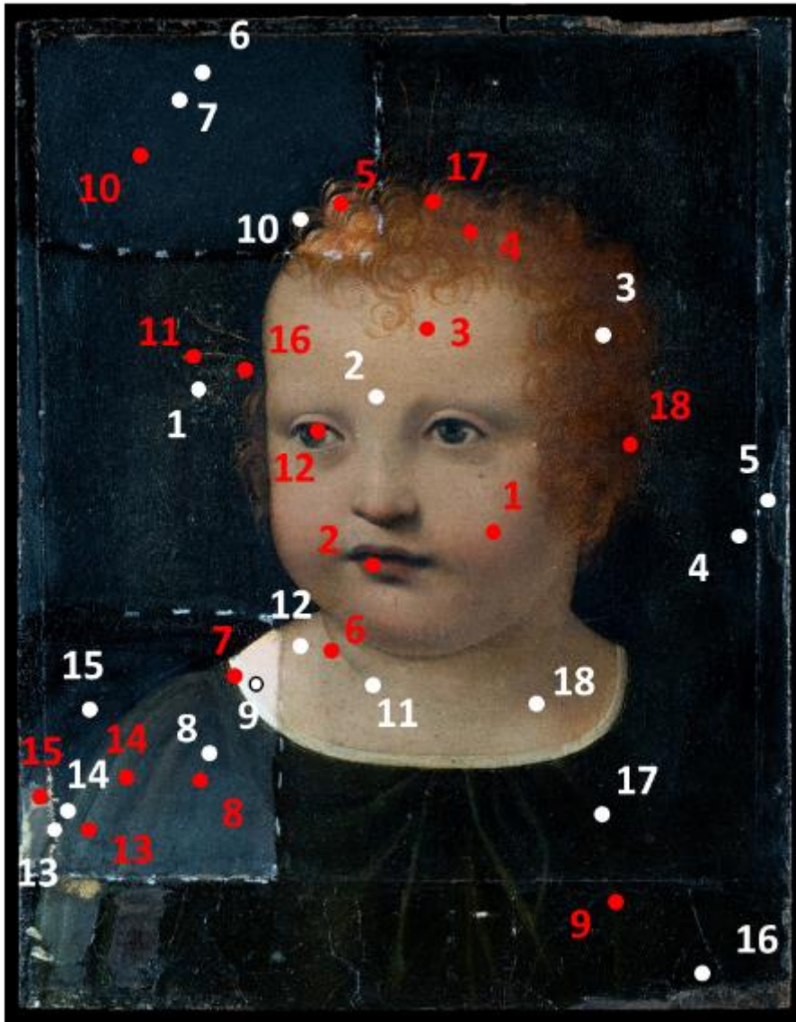
Fig. 1Sc: The Christ Child by Marco d'Oggiono: red dots indicate XRF, FORS, Raman and OM analysis areas; white dots refer to FT-IR analysis. As analyses were performed during restauration intervention, areas of cleaning proof areas are visible.
