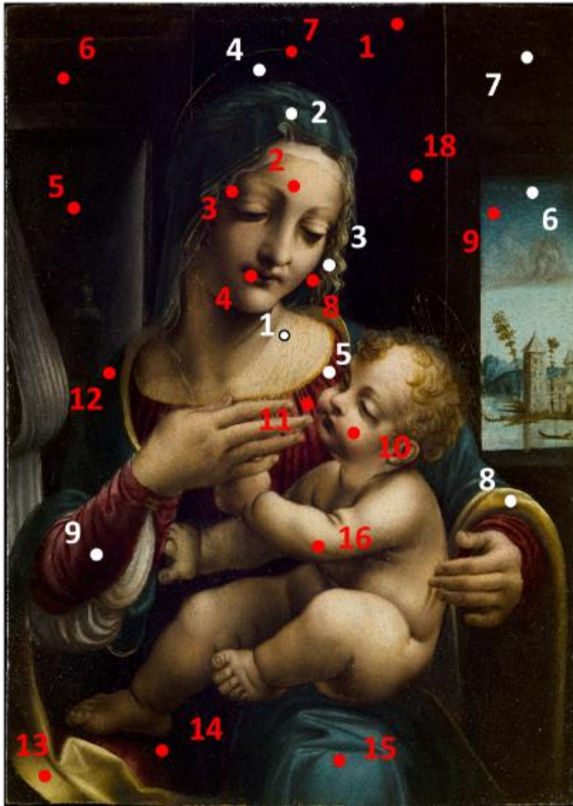
Fig. 1Sd: The Virgin and Child by Francesco Galli: red dots indicate XRF, FORS, Raman and OM analysis areas; white dots refer to FT-IR analysis.
