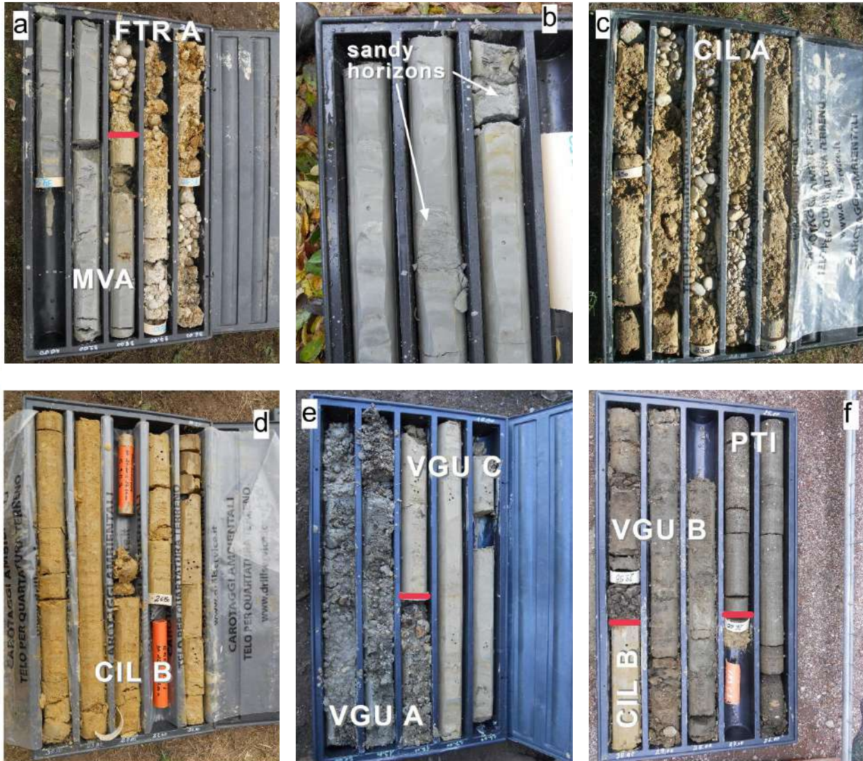
Examples of lithofacies from selected cores (bottoms and tops in the lower left and upper right, respectively; core box is 1 m-long), with main facies boundaries marked in red. a) Over-consolidated marine clay of The Monte Vaticano Formation (MVA; Pliocene) overlain by fluvial channel gravel (FTR A) of Fosso del Torrino Formation (Middle Pleistocene) in borehole 22 P (depth interval 40-35 m); b) dm-thick cross laminated sands intercalating the clays of MVA (detail from core of borehole 8 MS). Santa Cecilia Formation (Middle Pleistocene): c) channel gravel (CIL A) from borehole 2 MS (depth interval 15-10 m) and d) cross-laminated channel sand (CIL B) from borehole 16 MS (depth interval 30-25 m). e) The Valle Giulia Formation (Middle Pleistocene) in borehole 11 MS (dept interval 20-15 m): channel gravel (VGU A) passing upward to channel-abandonment fines of VGU C. Note the dark-grey hue of the VGU A sandy matrix, rich in ferromagnesian minerals; f) channel sand of the Santa Cecilia Formation (CIL B), overlain by grey overbank sand of VGU B lithofacies and by structureless ignimbrite of the Palatino Unit (PTI; Middle Pleistocene) from borehole 1 MS (depth-interval 30-25 m).
