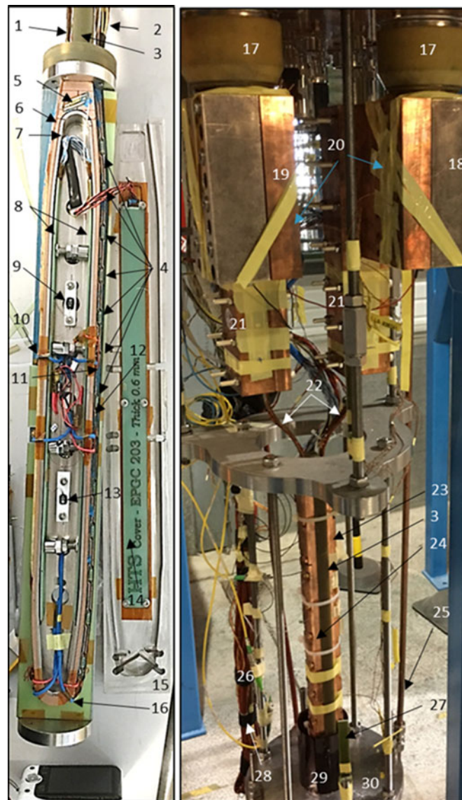
Fig. 13. (Left) Feather-M0.4 instrumented coil. (Right) Connections to test insert. Key: 1) Coil entry lead. 2) Coil exit lead, 3) Insulation between leads, seen in both pictures. 4) Part of CCS. Temp. Sensor array. 5) CCS temp sensor. 6) Cu coil former loop. 7) Magnet former support. 8) Pick-up coil sets. 9) Hall probe (a). 10) Spot heater #1. 11) Spot heater #2. 12) Position of fibre optic temp sensor in coil, adjacent to (11). 13) Hall probe (b). 14) Integrating field PCB coil. 15) Cover plate. 16) Spot heater #3. 17) 15 kA current leads. 18) -ve pole indium clamped joint. 19) +ve pole indium clamped joint. 20) Copper cryostat current lead to Roebel clamped connection adaptor plate. 21) Roebel cable clamped joints using indium sheets, Brass bolts. 22) Roebel cable link between Feather-M0.4 coil joint and cryostat current leads. With copper shunt & Kapton insulation 23) Coil joint box -ve pole. 24) Coil joint box +ve pole. 25) Variable temp gas supply pipe to bottom of magnet. 26) Fibre optic connector. 27) CERNOX temp sensor. 28) 4K helium auxiliary supply tube hidden in wires. 29) Kapton sheet ground insulation over Feather-M0.4 assembly that is inside the magnetic yoke. 30) Magnetic yoke top end plate.
