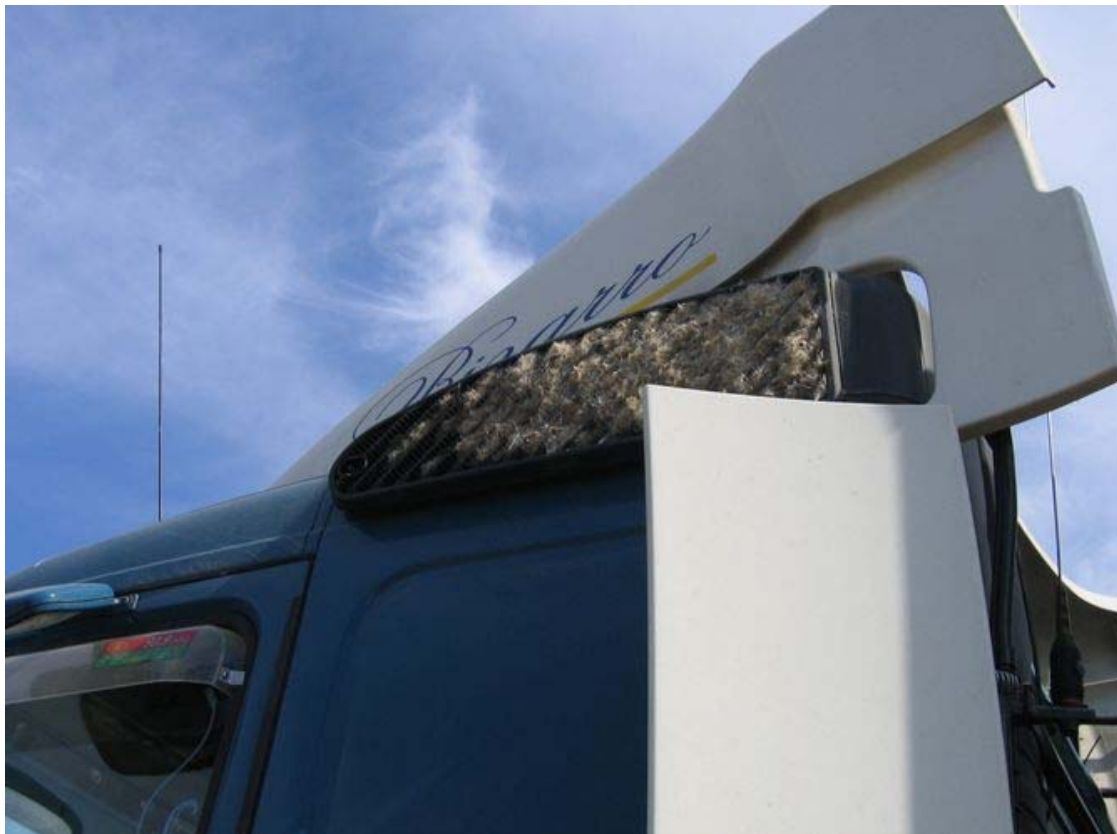
1-15: air filter occluded by pappi
