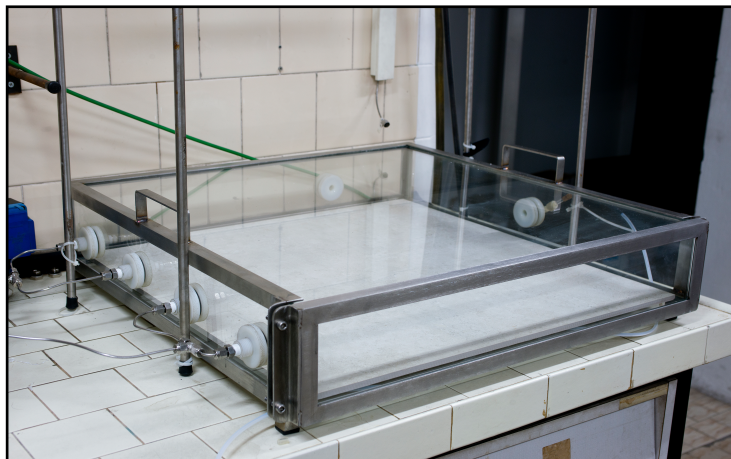
Fig. 2.18: Reactor containing the large \text{TiO}_2 ceramic tile ( 60 \times 60 \text{ cm}^2 )
