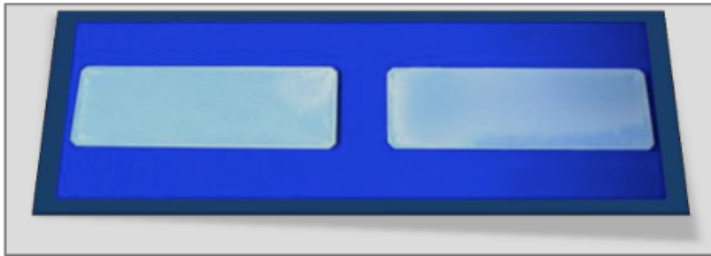
Fig. 2.12: \text{TiO}_2 deposited on glass as thin film, after the complete evaporation of 2-propanol.
