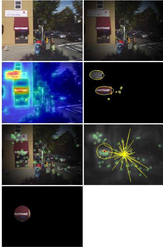
Fig. 4 The main representations that are obtained at the different levels of processing in the simulation (details in the simulation discussion, Sec. 4). In this case the given task \mathbf{T} is a “Look for text regions” task. From top to bottom, left to right: the original image \mathbf{I} ; the foveated image \hat{\mathbf{I}} obtained by setting the initial FOA \mathbf{r}_F(0) at the centre of the image; the priority map \mathbf{L} ; selected proto-objects parametrised as ellipses \theta_p(t) ; the interest points O(t) sampled from proto-objects; the sampling process of candidate FOAs \mathbf{r}_{new}(t+1) (Eq. 17) and the selection of k -th candidate point which maximises the expected reward E[R_{\mathbf{r}_{new}}] (the big circles covers the points within \mathcal{I}_V^k ); the sampled FOA \mathbf{r}_F(t+1) . All maps are depicted at the same resolution (HR) of the original image \mathbf{I} for visualisation purposes. Value map initialisation follows the procedure illustrated in Fig. 5 below
