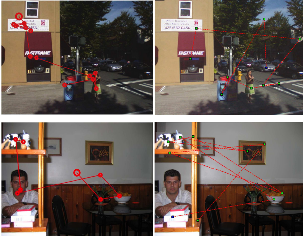
Fig. 1 Scan paths generated by free viewing pictures embedding semantic objects (faces, text). Left: scan paths obtained eye-tracking a human observer. Right: scan paths simulated using the Itti et. al model [54] as implemented in the latest version of the saliency tool box downloaded from http://www.saliencytoolbox.net using the default parameters.
