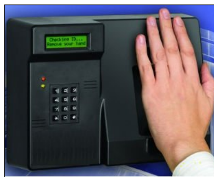
Figure 2.14: Example of a palm vein scanner, able to capture the vein pattern of the hand [61].
