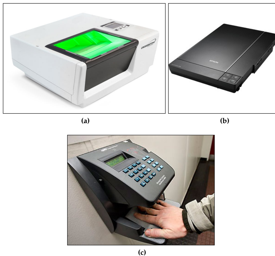
Figure 2.13: Example of palmprint acquisition devices: (a) optical device [58]; (b) flatbed scanner [59]; (c) CCD-based device [60].
