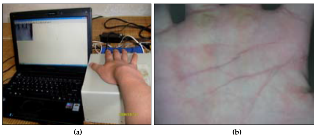
Figure 4.23: The contact-based two-dimensional CCD acquisition device described in [327]: (a) the device; (b) example of acquisition.
