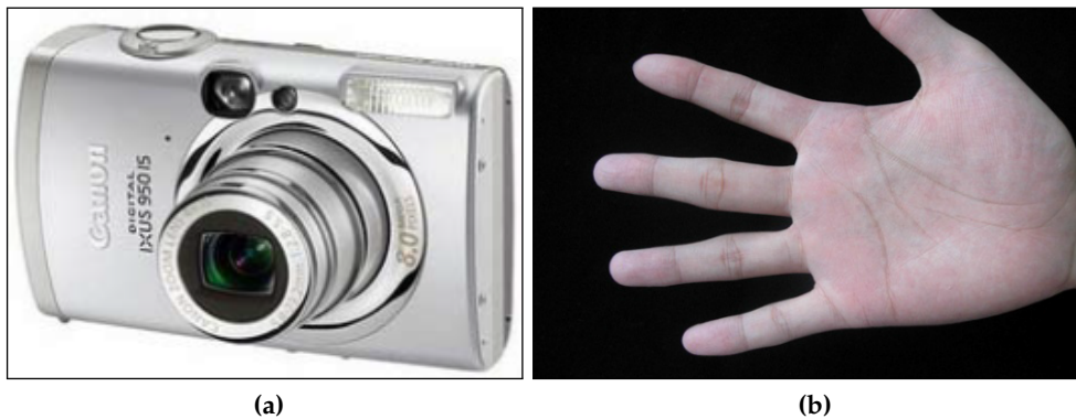
Figure 4.12: Example of a CCD camera for contactless, two-dimensional palmprint acquisitions [228]: (a) the device; (b) the corresponding sample.
