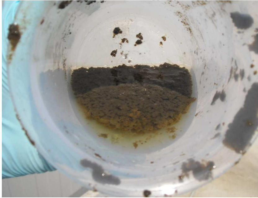
Figure 4.20. Dimension of the aggregates after flocculation.
