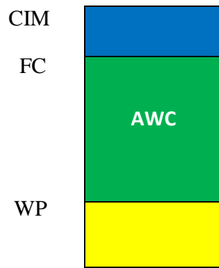
Figure 5. The scheme of tank approach model: maximum water capacity (CIM), field capacity (FC) and wilting point (WP)
