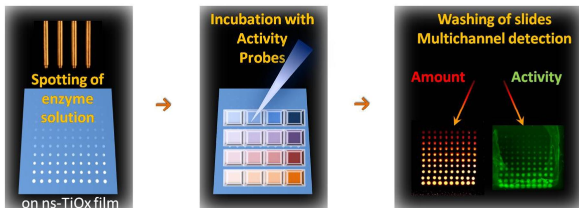
Fig. 2.3.3.1. Scheme of the microarray-based assay for high-throughput assessment of the activity of physisorbed enzymes. Left panel: Fluorescently labeled enzymes are physisorbed by means of arraying on the material surface of interest. Middle panel: The immobilized enzyme arrays are incubated with various concentrations of fluorescent activity probes for a range of time intervals. Right panel: Slides with arrays are blocked, washed and scanned to detect the adsorbed amount, as well as the activity in separate fluorescence channels.
