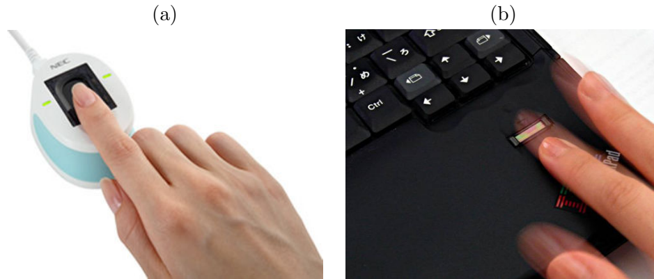
Figure 4.12: Examples of fingerprint acquisition sensors: (a) area scan sensor; (b) swipe sensor.
