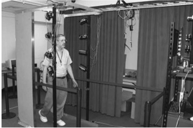
Figure 3.2: Example of iris recognition systems based on images captured at a distance on the move [132].
