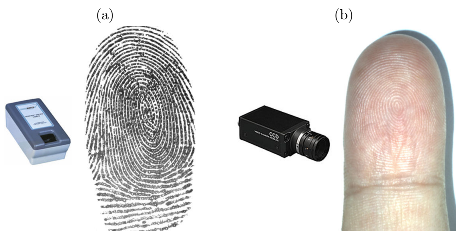
Figure 4.18: Examples of fingerprint images captured using a contact-based sensor and a CCD camera: (a) contact-based image; (b) contactless image. Contactless fingerprint images are more noisy and present a more complex background.
