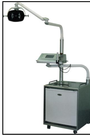
Fig. 14 – Lasericemed-cryoRx - The instrument exists in two configurations, a fixed one, mainly used in medical studies and a portable one used for home purpose or directly in the sport field. The devices differ only for the appearance; the laser sources and the powers used are the same in both versions. There is also a portable version for veterinary purpose which is used primarily for horses treatment using a different configuration of laser capable of eliminating the problem of hair in the passage of the drug. Picture modified form: https://www.box.com/s/anr9knr2g9oyv2yb0fj .
