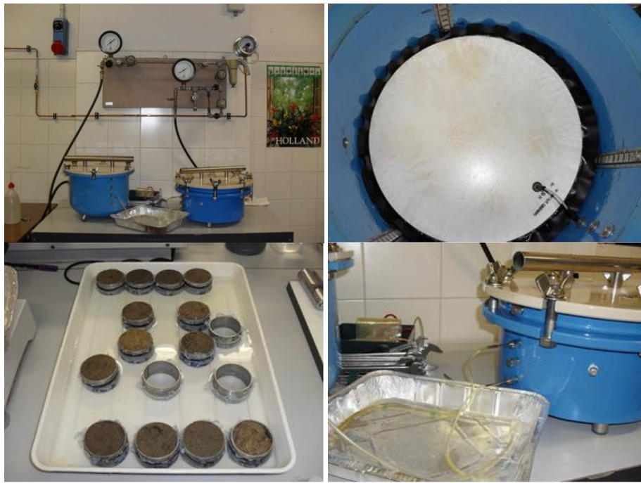
Figure 5.1 Plate of Richards and the determination of retention curves in the laboratory
