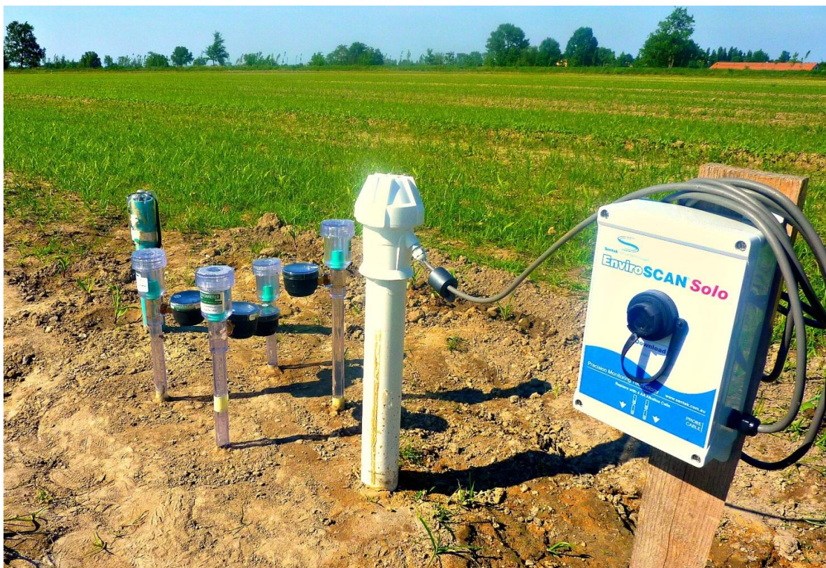
Figure 4.2 Different instruments installed in each site for soil water status monitoring
