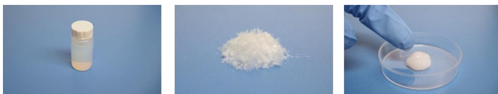
Figure 5 1% dispersion (a), freeze-dried powder (b), and 3.5% CNs gel (c), from left to right. The yellow parts caused by the light of the lamps.
