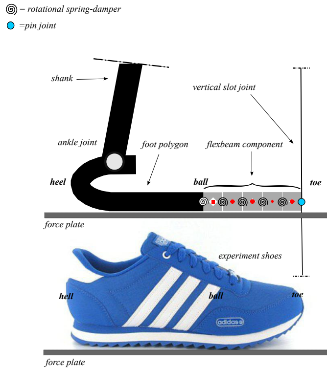
Figure 3.2: Detailed foot-ground interface of the model, which represent the feet of the subject. The five final segments linked by using springs allowed to better reproduce the natural movement of the foot during plantar flexion movement. The length of the foot segment was calculated measuring the length of the shoe used during the experiment. The vertical slot constraint attached at the toe was created to avoid sliding during the push-off phase of the jump.
