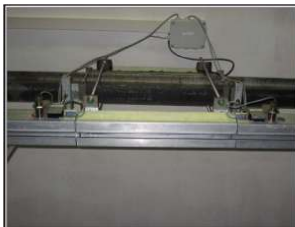
Figure 3.52 - System photocell-reader to read the hooks and to detect the advancing direction of the bovine sides.
