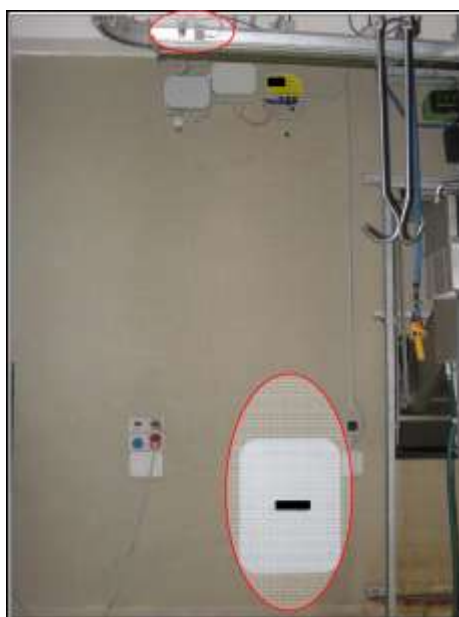
Figure 3.50 - Combining system of the microchip to identify animal and microchips on the hooks.
