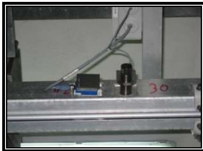
Figure 3.53 - System EMS reader-photocell in the dissection area.
