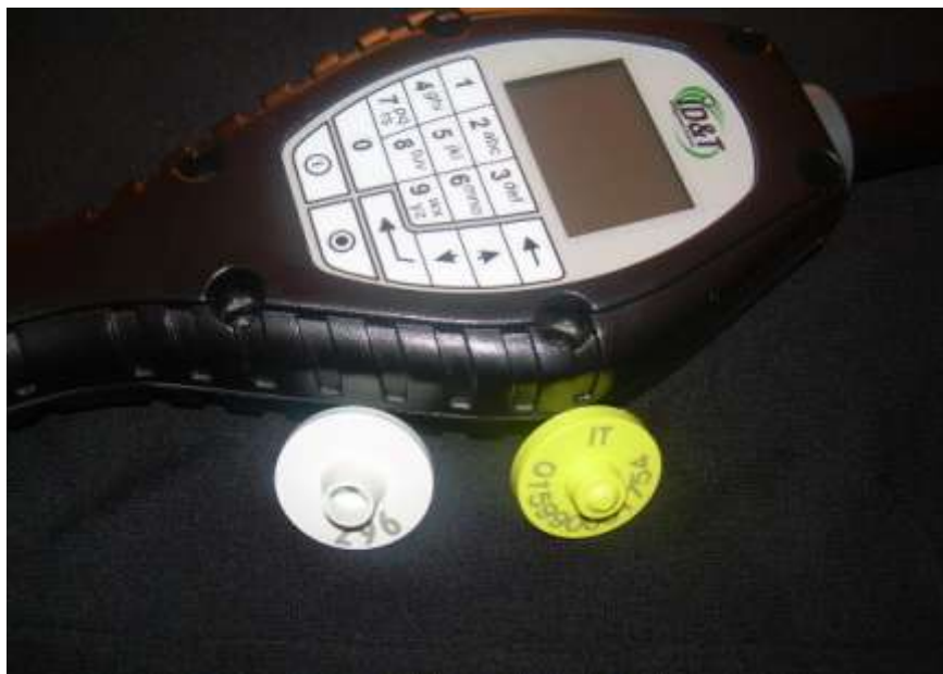
Figure 3.28 – Handheld reader HHR3000 Pro (ID&T – Norway) and e-tags used in the test
