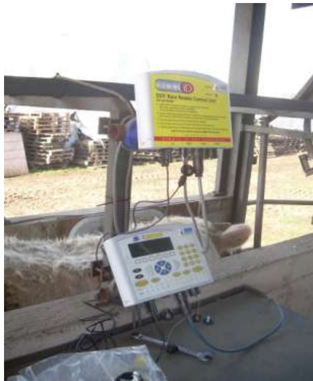
Figure 3.34 – RFID reading system and weighing scale.
