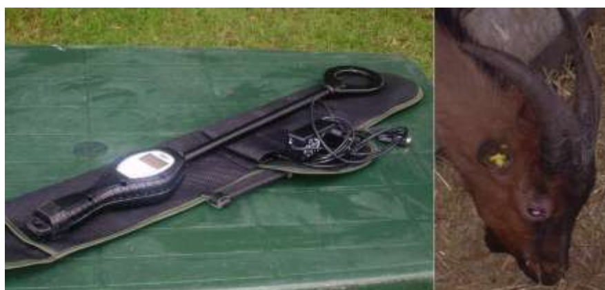
Figura 3.48 - Left: handheld RFID reader with integrated and programmable handheld; right: e-tag to the ear of an animal.
