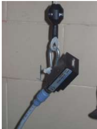
Figure 3.54 - Device for reading/writing food RFID tags to be put inside the vacuum-packages.
