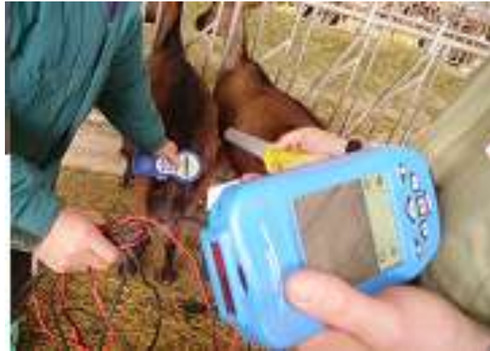
Figure 3.45 - Acquisition system of individual animal data at the enterprise level through RFID reader- PDA system.
