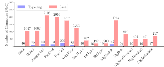
(b) A visualization of the NoC reduction achieved by implementing a type system using Typelang for some Neverlang artifact compared to a traditional Java-based approach. This figure illustrates how the use of Typelang leads to significant simplification, with a reduction of approximately 93.48%.
