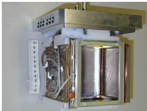
Figure 6.3: Schematic view (left) and picture (right) of the MCP detector of PRISMA. Reprinted from Ref. [149].
