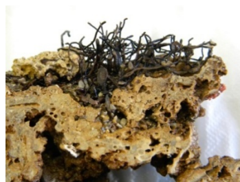
Fig. 2. Cross-section of calcarenite with roots system above
