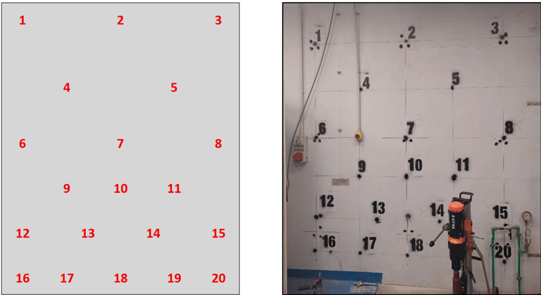
Fig. 5. Schematic representation and real outline of second sampling net.
