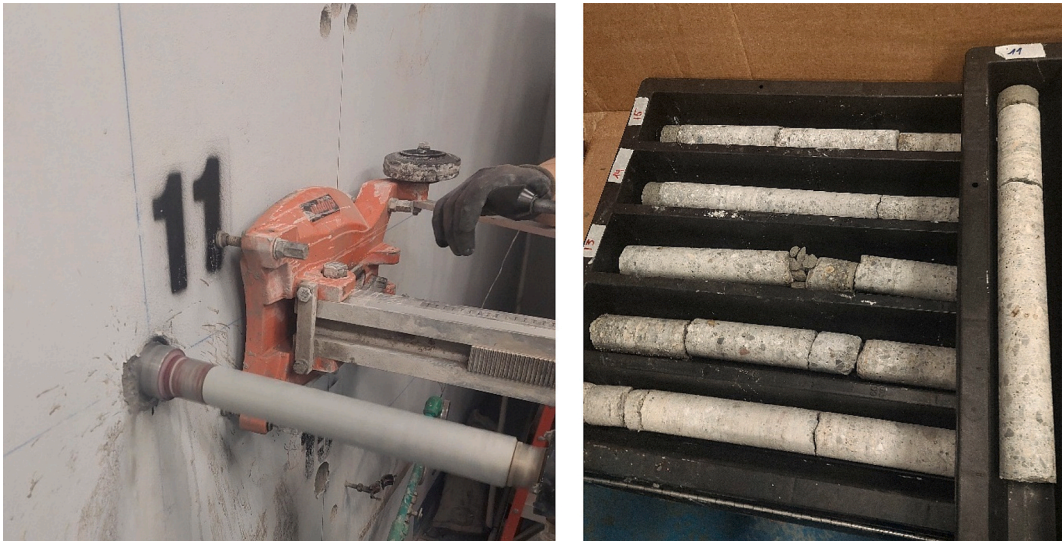
Fig. 6. Sampling and sampled concrete cores.
