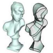
Fig. 31. A comparison between our field-aligned patch layout with the Voronoi partition with Lloyd relaxation and Variational Shape Approximation [Cohen-Steiner et al. 2004]. The proposed method results in a better approximation of the target geometry, when each patch is discretized in a fully developable ruled surface, for a similar total length of the cuts.
