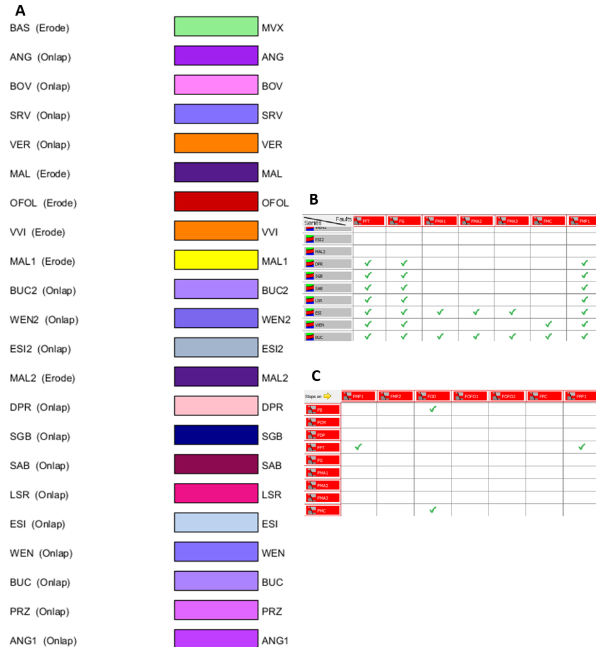
Fig. 4.10 A: geological pile of the Val Sabbia 3D model (the acronyms of the formations are given in Fig. 4.1). B: a detail of the table that specifies faults and series relationships. C: a detail of the table linking faults with other faults.
