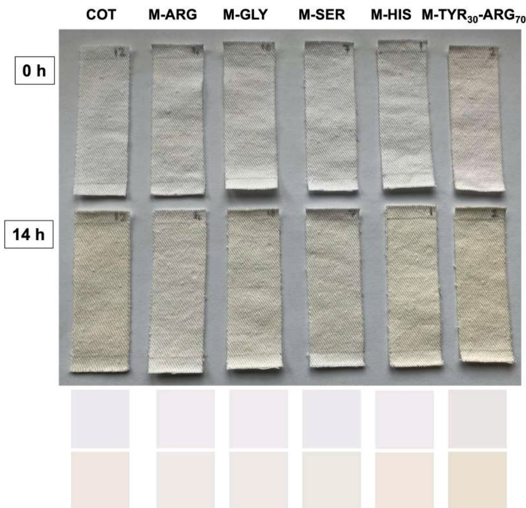
Fig. 3. Digital pictures of untreated and PAA-treated cotton fabrics after 0 and 14 h photoaging (upper panel); simulated colors of photoaged cotton samples based on the determined colorimetric parameters (Section 2.5) (lower panel).
