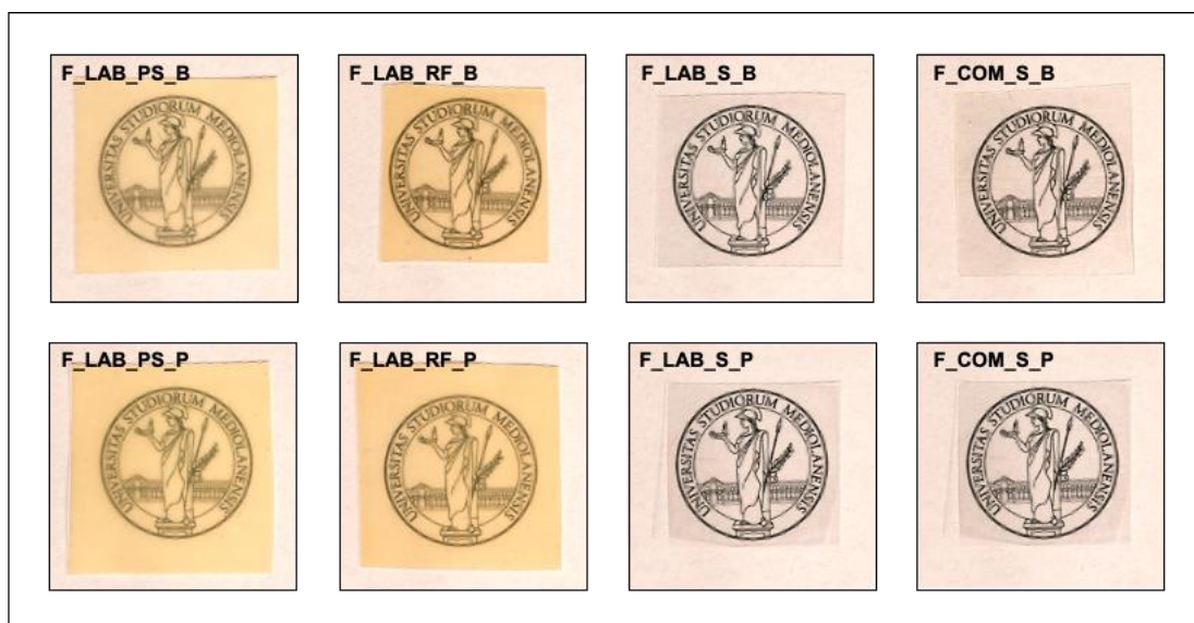
Fig. 6. Transparency of experimental films of the present study. The films were individually placed on a white paper to cover the logo of University of Milan (diameter of 3 cm) and photographed.
