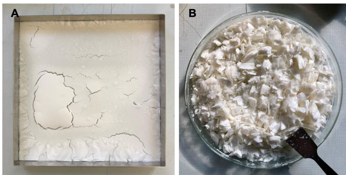
Fig. 1. Appearance of NaCas powder just after freeze-drying (panel A) and after grinding (panel B).
