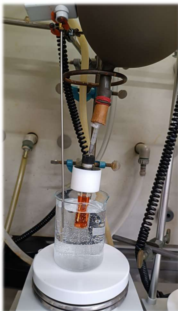
Figure 27: Electrochemical set-up for secondary chiral amines homo-coupling
