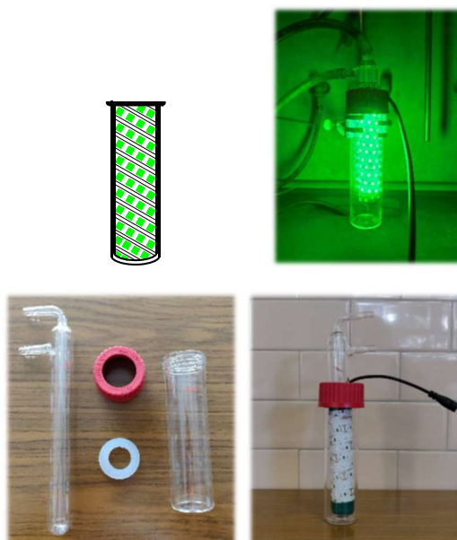
Figure 42: A) Water-cooled photoreactor scheme. B) Assembled photoreactor (on). C) Assembled photoreactor (off). D) Unassembled photoreactor (without LED strip).
