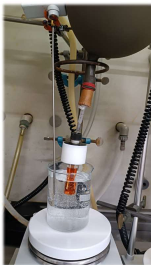
Figure 41: Electrochemical set-up for the dehydrogenative homo-coupling of compounds 94a-e
