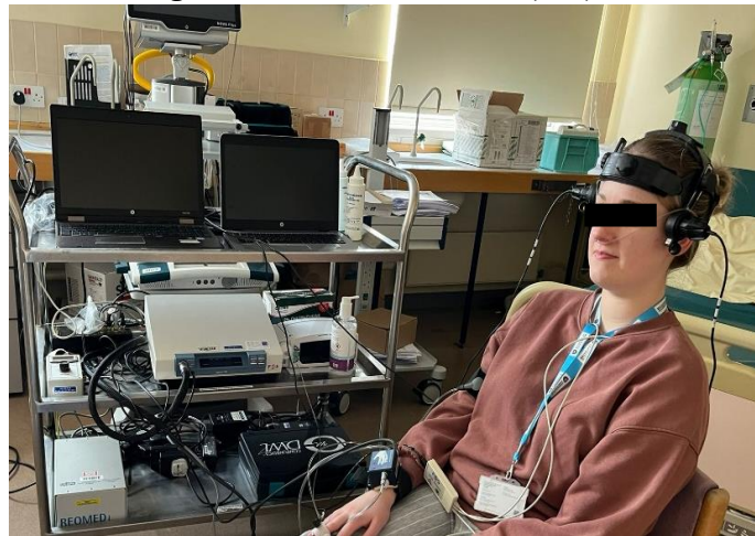
Figure 3.3 Experimental setup for TCD, capnography, ECG and BP recordings at the University of Leicester's Cerebral Haemodynamic in Ageing and Stroke Medicine research laboratory. Courtesy of Lauren Walker.
