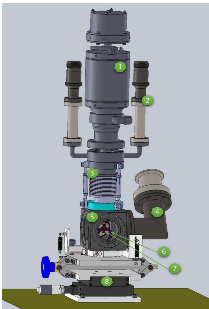
Figure 3.6: Image of the cooling system with numbered pins to highlight the key components: (1) the closed-circuit cryostat for cooling the sample, (2) the electrical feedthrough with 6 pins mounted on a DN16CF flange for heater power supply and temperature reading (3) a bellows on a DN40CF flange with 6 manually controllable degrees of freedom for sample manipulation (4) a flange for pumping (5) a vacuum chamber for housing the sample and the electromagnet (6) the electromagnet, (7) a sample holder, and (8) a mechanical base with five axes of movement (X, Y, Z, chi, and theta) for positioning the entire setup relative to the laser beam. Image courtesy of A. Fondacaro.
