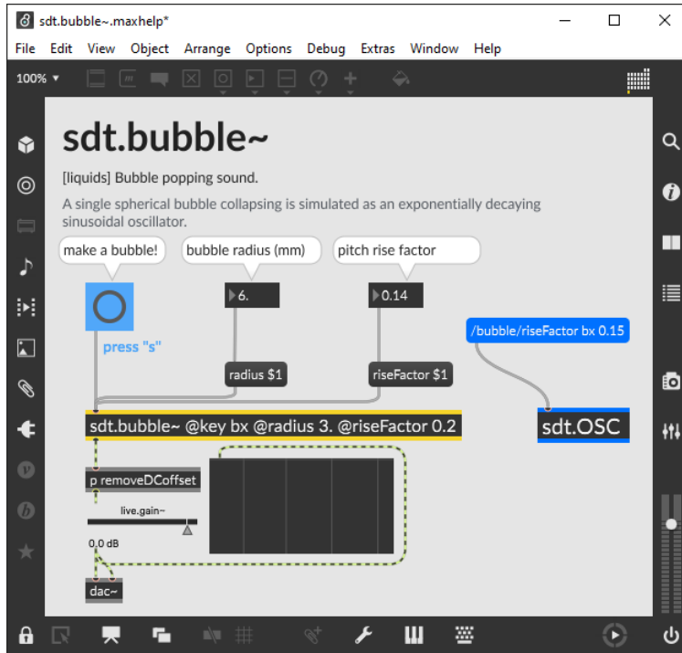
Figure 20: Example of the Max help patcher for sdt.bubble~ objects (in yellow), with the addition of the sdt.OSC object and an OSC message (both in blue) to set the “rise factor” parameter.
