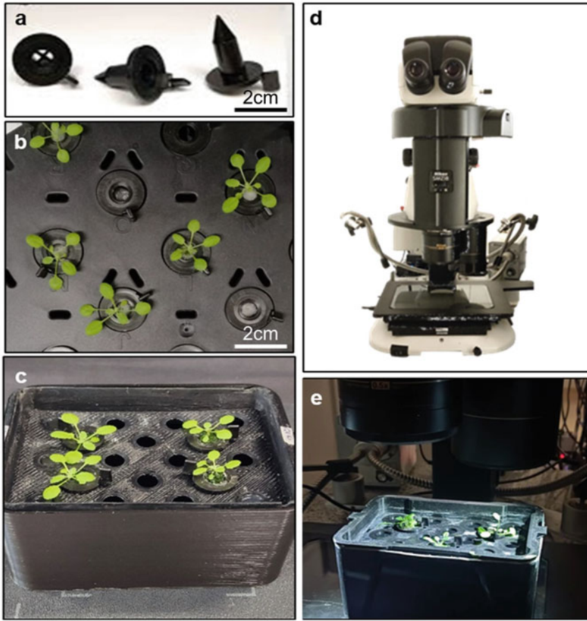
Fig. 2 Experimental setup for in vivo mesoscopic imaging. (a, b) Plant-holders for plant growth in hydroponic. (c) 3D-printed hydroponic system. (d) Nikon SMZ18 fluorescence stereo microscope. (e) Whole plant imaging for unperturbed in vivo acquisition
