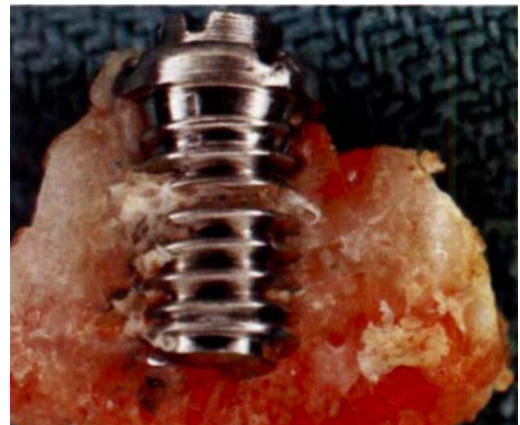
Figure 12 Implant inserted in dog bone after 32 weeks from insertion and 16 weeks from loading. (Branemark 1969)
