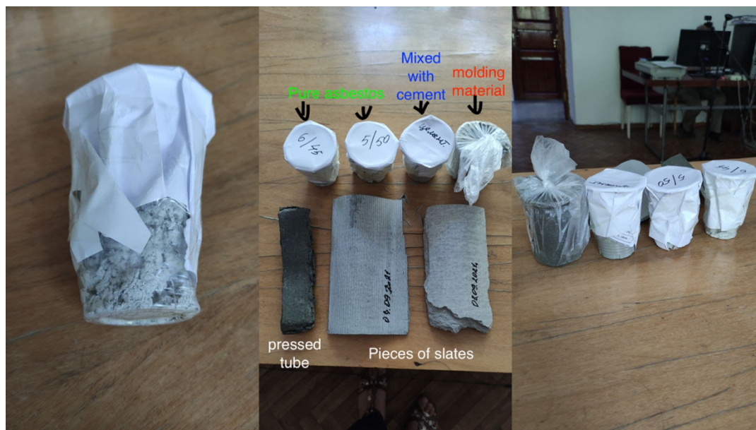
Figure 3. Bulk asbestos material and asbestos-containing products. Source: photo taken by Z.Kurzunbaeva.
