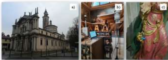
Figure 1. a) Street view of the Sanctuary; b) P-Dust Monit and MQA; c) Diffusive passive samplers
