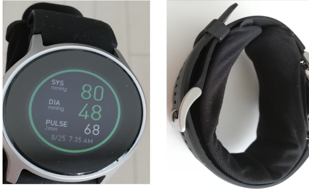
Fig. 1. An Omron wearable blood pressure monitor HeartGuide™. Left: blood pressure and heart rate readings on the display. Right: the wristband contains a cuff that will be inflated during a measurement.
