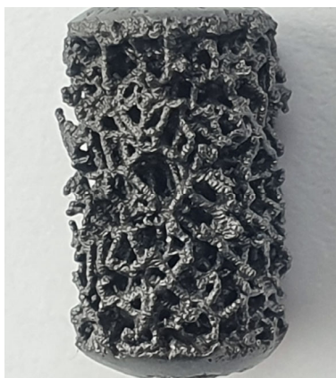
Figure 1. The macrophoto shows a 3D scaffold with a native surface. This prototype, 6.2 mm in diameter and 11 mm in length, was produced for the in vivo study experiment.
