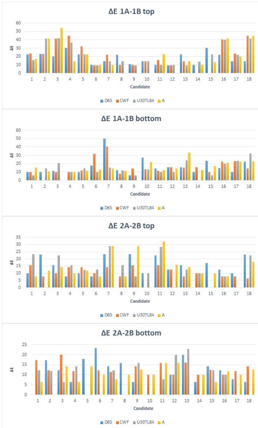
Figure 2. \Delta E values for each candidate and each illuminant for configurations; a) \Delta E 1A and 1B top b) \Delta E 1A and 1B bottom c) \Delta E 2A and 2B top d) \Delta E 2A and 2B bottom.
