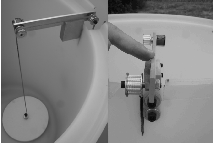
Fig. 2: Floating level system.
