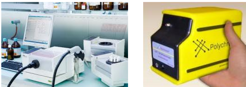
Figure 3.51: Master (right) and slave (left) spectrometers used in the calibration transfer.
