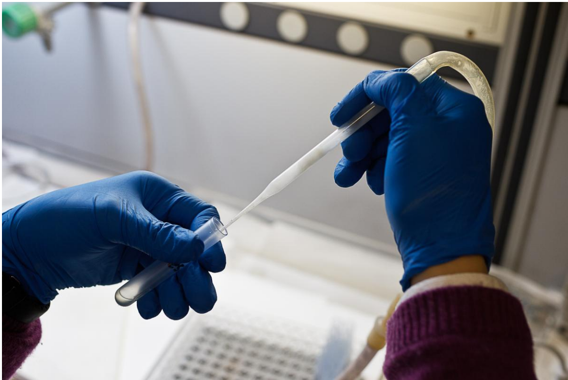
Figure 5. Aspiration of the supernatant from a tube before analysis of cortisol in the gamma-counter
