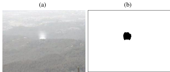
Fig. 1. Example of smoke frame with pixelwise segmentation: (a) original frame; (b) segmented image.
