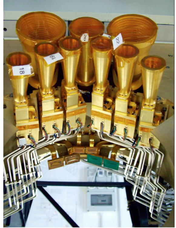
Fig. 12. Picture of nine of the eleven feed horns and associated OMTs, FEMs, and waveguides before integration of the HFI front end. The six smaller feeds in the front supply the 70 GHz channels. In the back row, the two 30 GHz feeds flank one of the 44 GHz feeds. Visible are part of the twisted Cu waveguide sections and the reference horns (protected by a kapton layer): for the 70 GHz FEMs they are embodied in the FEMs, while for the 30 and 44 GHz they are flared waveguide sections.
