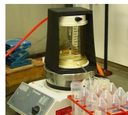
Figure (8). Ultra filtration cell for 50mm filter paper.
