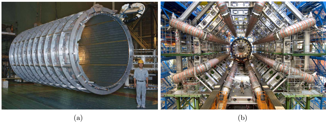
Figure 1.12: Photos of the magnets of the ATLAS Experiment: (a) the solenoid and (b) the barrel toroid.
