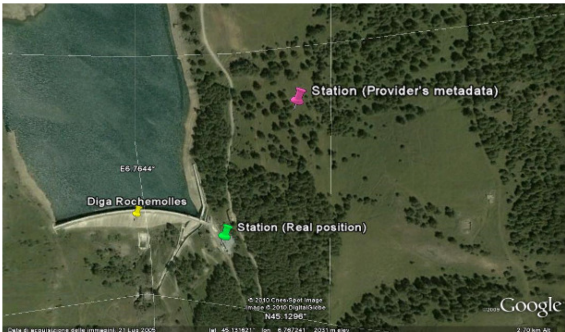
Fig.26 Yellow placeholder: Diga Rochemolles; purple placeholder: station position as labelled by provider's metadata; green placeholder: real station's position (Google Earth™)
