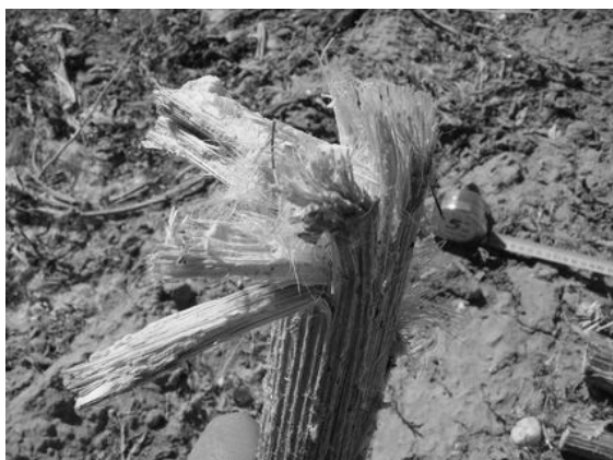
Figure 10: rotating blades scraped cut
