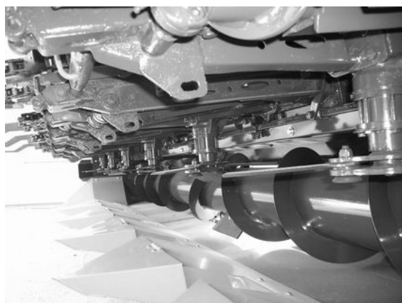
Figure 3: squeezing rolls and rotating blades
