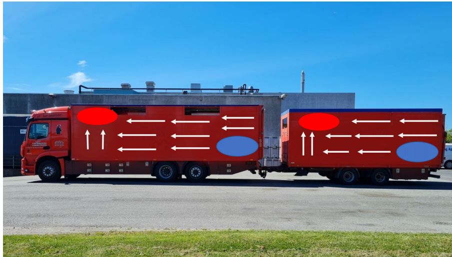
Figure 4: Predominant patterns of air flow (white arrows) in a moving passively ventilated vehicle. The red area in the front indicates where air heated by the animals accumulates and the blue area show the colder rear spots. Adapted from picture taken by (Adapted photo taken by Magnus and Morten Bach Sørensen, Simsted Vognmandsforretning)
