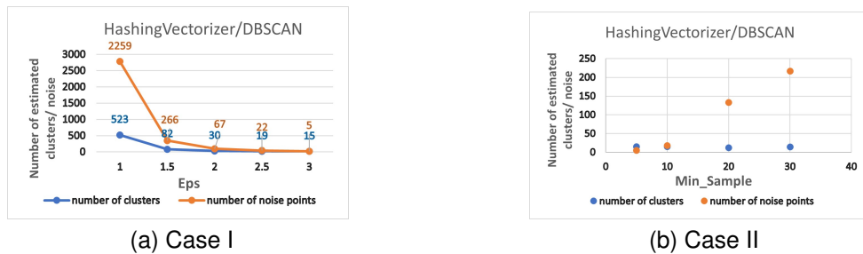
Fig. 3. The estimated number of clustering and noise points in term of Eps and Min_samples are plotted respectively as case I and case II, using the HashingVectorizer method in vectorizing and DBSCAN for clustering task.
